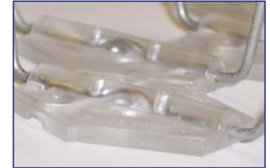
Wires insert moulded into base
